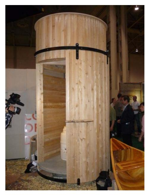
Also spectacular is the Fons, "providing for responsible sanitation." this round tower has a composting toilet, a sink, a shower, and a rainwater collection system and cistern at the top. A very elegant curved sliding door rotates around the unit.
